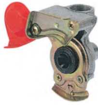
Palm-Couplings for Two Line System Confusion Preventing Type Automatic Type (with valve) Withworth 1/2 inches also available
